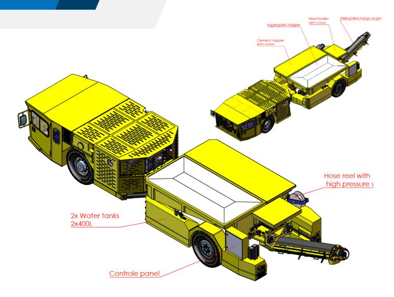
The Hencon TransVers Low Profile Batch Mixer has been designed for the preparation of concrete mixtures.
